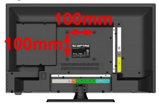
Mounting Specification: 100mm x 100mm using 4 screws (not included) at size M4. The mounting holes are 20mm deep.
